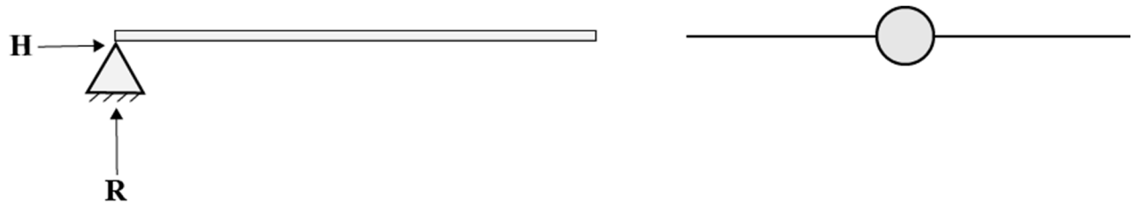
Fig. 3.2: Hinged Support and Hinged Joint
